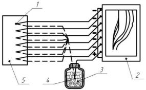
**Figure 3 Schematic diagram of the device for measuring temperatures using microtherm battery.** Note: 1 - hot jig, 2 - multipoint electron potentiometer, 3 - Dewar dish, 4 - total cold junction, 5 - investigated object.
