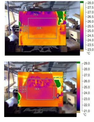
Figure 7 Thermal imaging of the injection unit. Note: a) a new roll construction; b) the existing roll construction.
