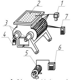
**Figure 2** Scheme of injection nozzle for determination of temperature fluxes and power. Note: 1 - thermal imager; 2 - medium (dough); 3 - roller working bodies; 4 - tachometer; 5 - electric motor; 6 - watt meter; 7 - potentiometer.
