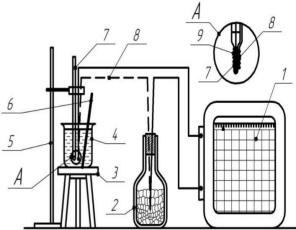
Figure 4 Scheme of installation for calibration of thermocouples.
