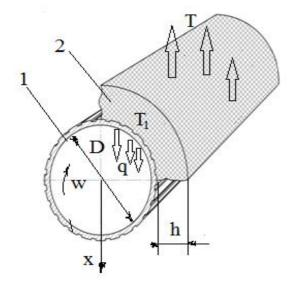
Figure 1 Scheme of impulse friction contact. Note: 1 - roll working body, mm; 2 - medium (dough); T - constant temperature;  $T_1$  - is the temperature on the surface of the frictional contact.
