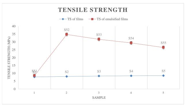
**Figure 6** Comparison of tensile strength (TS) of chitosan and emulsified edible films. Note: \*Si = Aloe vera concentration; S1i = Beeswax concentration; S1 = 0%; S2 = 5%; S3 = 10%; S4 = 15%; S = 20%; S51 = 0%; S52 = 0.5%; S53 = 1.0%; S54 = 1.5%; S55 = 2.0%.
