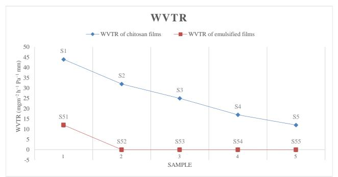
**Figure 4** Comparison of water vapor permeability of chitosan and emulsified edible films. Note: \*Si = Aloe vera concentration; S5i = Beeswax concentration; S1 = 0%; S2 = 5%; S3 = 10%; S4 = 15%; S = 20%; S51 = 0%; S52 = 0.5%; S53 = 1.0%; S54 = 1.5%; S55 = 2.0%.
