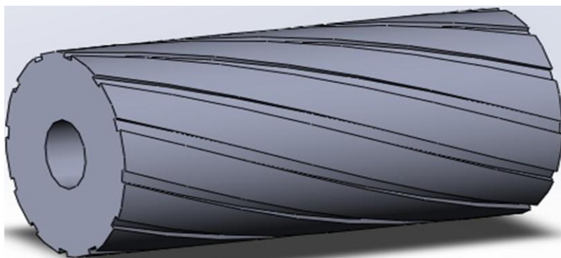
Figure 3 New Spiral roller working body design.
